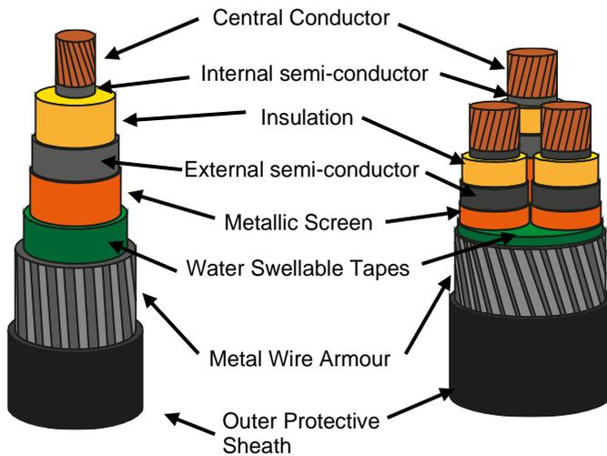
**MV Cabling:** Three single core cables or one three-core cable
